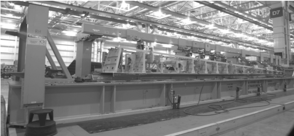
Figure 4a – Empennage Assembly Tool used for acceptance test
